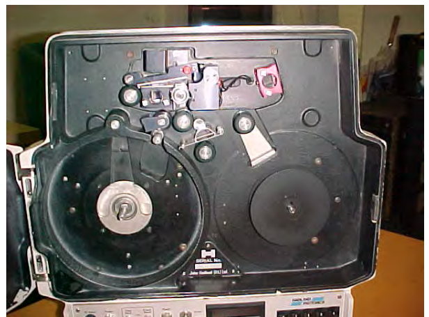
The Hadland Hyspeed was capable of 10000 frames per second full-height, 40000 ¼ height
