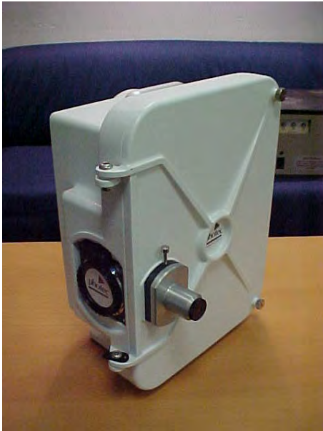
Photoc – 10,000 fps full height and up to 40,000 with ¼ frame prism conversion.
