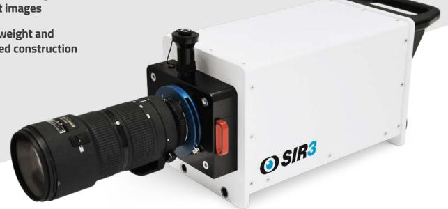
The Specialised Imaging SIR3 Framing Camera offers up to 2 high resolution images, 100µs apart. Fully flexible intensified CCD sensor provides control over interframe time, gain and exposure.
