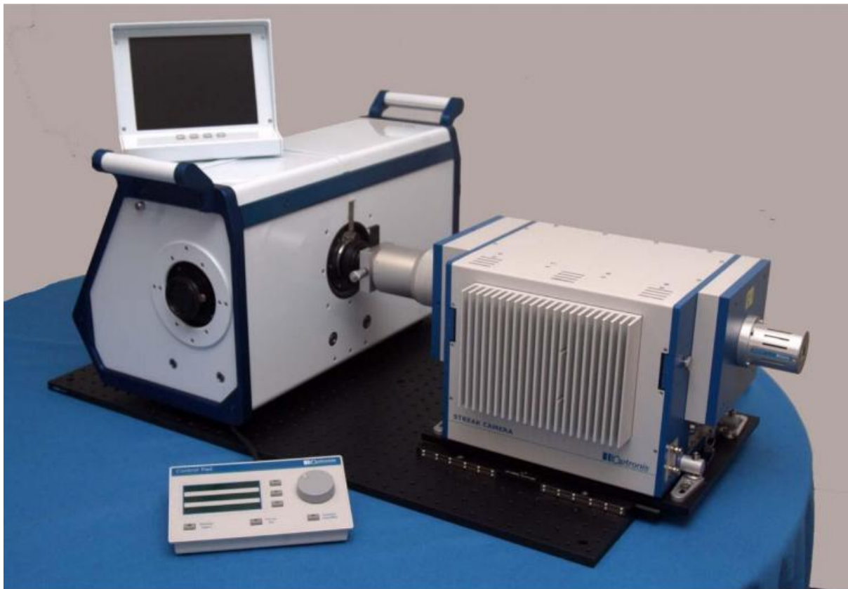
Fig 1. The Specialised Imaging Combined Framing and Streak Camera System incorporating a Specialised Imaging SIM 16 Channel Framing Camera coupled with an Optronics SC10 Streak Camera.
