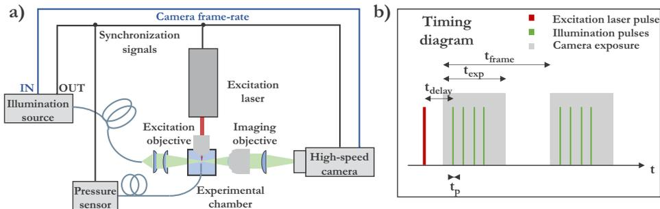
**Fig. 1.** a) Experimental setup schematic drawing, and b) timing diagram. Synchronization timing jitter between the excitation laser pulse and the camera exposure was approx. 1 ns, and well below 1 ns between the camera exposure signal and optical illumination pulses.
