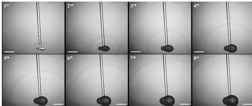
**Fig. 5.** Shock wave propagation following a single LIB event shown on 8 consecutive frames from the Kirana camera at 5 MHz, capturing the same shock wave at 32 different times due to burst illumination. The FOPH is visible in the images, providing a simultaneous shock wave pressure and time-of-flight measurement at its tip position. Scale bars equal to  $500 \text{ }\mu\text{m}$ .
