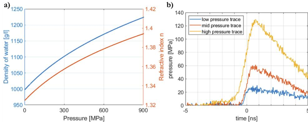
**Fig. 4.** a) Refractive index and density of water, plotted versus pressure, and b) sample pressure traces from the FOPH, showing shock wave arrival at 0 ns.
