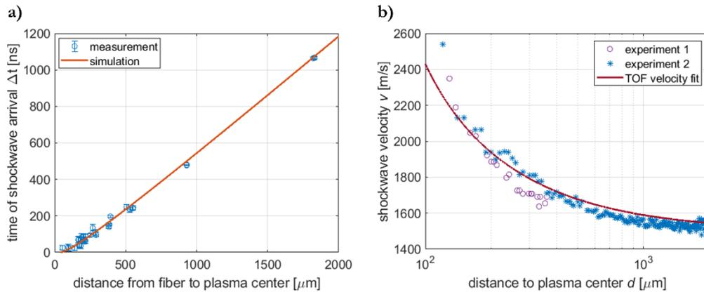
**Fig. 7.** a) Time-of-flight (TOF) measurement from pressure sensor with the corresponding velocity distribution integral, and b) shock wave velocity measurements from both experiments (camera-based) with the TOF velocity distribution plotted as a continuous line. Bubble sizes were maximal for both experiments, 1.35 mm and 1.67 mm, respectively.
