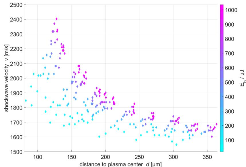
**Fig. 8.** Shock wave speed measurements for different excitation laser energies within Experiment 1, color coded for the corresponding bubble energy  $E_b$ .
