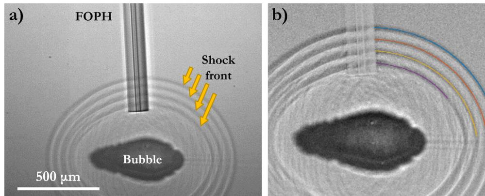
**Fig. 6.** a) Shock wave propagation near the initial LIB region and pressure sensor (FOPH) positioned nearby. The excitation laser pulse propagated from right to left. b) Improved contrast, background removed, and shock wave front recognition result. Different colors show the recognized position of the same shock wave front at different illumination times.
