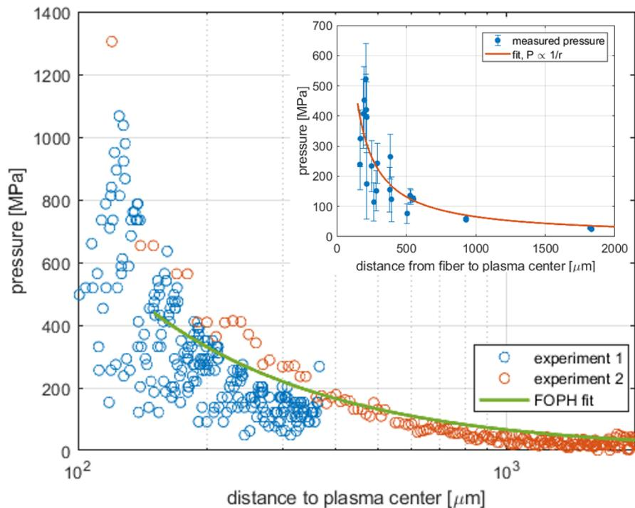
**Fig. 9.** Shock wave pressures obtained from camera-based shock wave velocity measurements (blue and orange circles), values converted using Eq. (1). The data presented is from both experiments and for all bubble sizes, including the fit on measured pressures from FOPH. Inset: Pressure measurement from FOPH with the corresponding  $1/r$  best fit.
