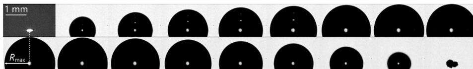
**Fig. 3.** Time series over the entire first oscillation cycle of the bubble developing from the plasma, the time between two frames is 10  $\mu\text{s}$ , i.e. a span of 170  $\mu\text{s}$  is covered in this series. The first image shows the plasma, and the background is presented darker for clarity. Only a section of the spherical bubble is shown.
