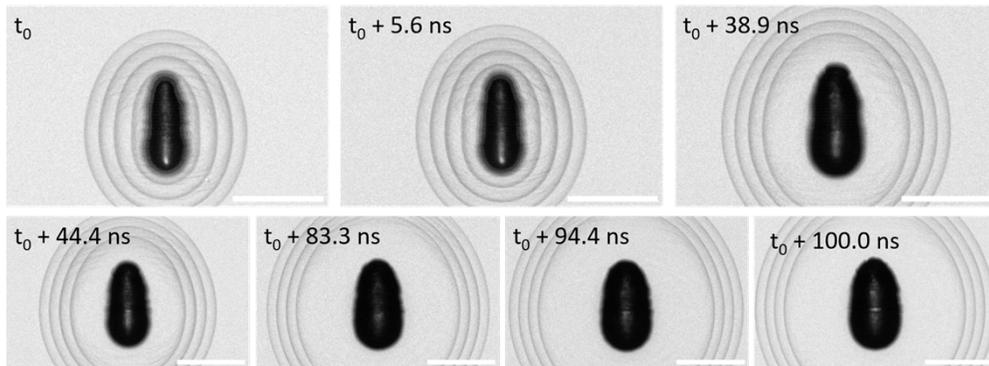
**Fig. 2.** Shock wave imaging with four pulse burst illumination at different time delays after the LIB event, showing 7 individual LIB events. The  $t_0$  denotes the initial nonzero delay. Scale bars are equal to 200  $\mu\text{m}$ .
