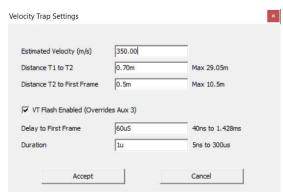
This standard feature of a built in real time velocity trap provided by the KIRANA camera system significantly reduces the likelihood of missing extremely fast events such as cracking of a ceramic plate or back face deformation of a carbon fibre panel when hit by a projectile of variable velocity.
