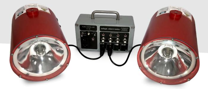
The Specialised Imaging AD500 Flash system offers the flexibility of up to four controllable high intensity flash heads for use in scientific and industrial environments. 500J Flash head with 2ms duration Up to four independent flash heads 40s recycle time Trigger options - short or positive edge
